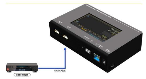
When MS-5005 set as receiver, it can verify HDCP of video player or other DUT (Device Under Test). MS-5005 provides three options (HDCP 1.4 / HDCP 2.2 / no HDCP) for users to select and confirm the HDCP authentication of DUT.
