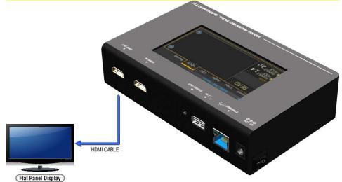
After making the physical connections between MS-5005 and the display device. User can select different generator function to display on the sink device under test.
